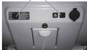
Electrical Access Panel (Fuses/Main Disconnect Switch)
