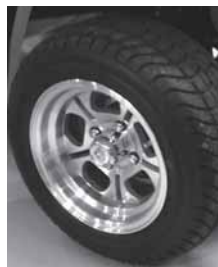
12-inch Turf (accessory) 95 ft. lbs. (128 Nm)
